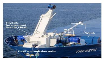
Currently, SkySails is equipping a series of three Rhine class ships being built for Wessels at the Komarno shipyard in Slovakia with its wind propulsion system. The MV "Theseus" has become the first ship in this series to be equipped with the latest-generation SkySails-System, into whose development were channelled the many important lessons learned during pilot testing.
