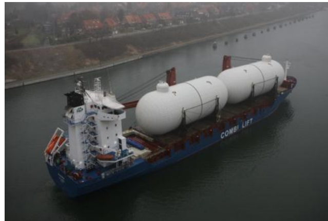
Transportation of Stainless Steel cargo tanks for a 7,500 m 3 LNG carrier on a heavy lift carrier to a shipyard in Europe
