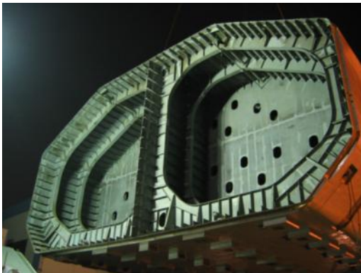
Cargo tanks type A for a 23,000 m 3 Fully Refrigerated LPG Carrier
