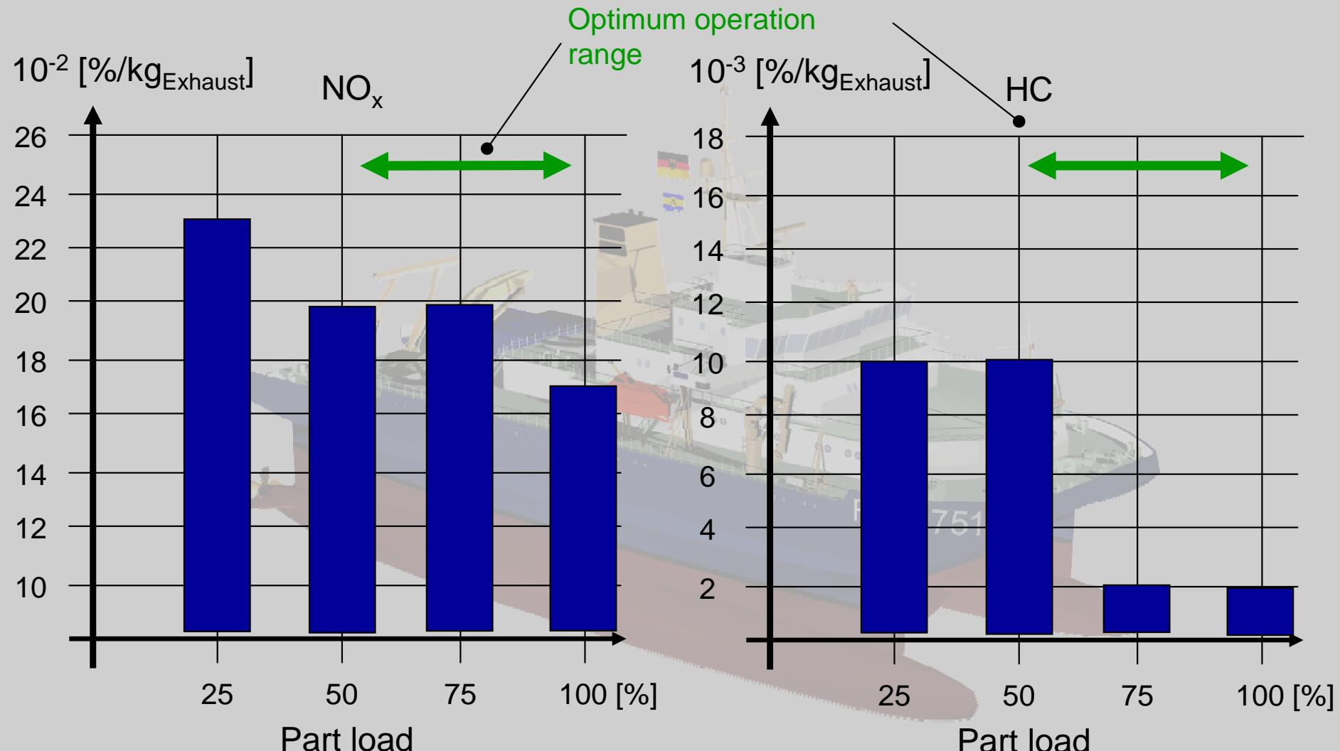
Values for orientation based on measurement results at a (MDO) diesel engine
