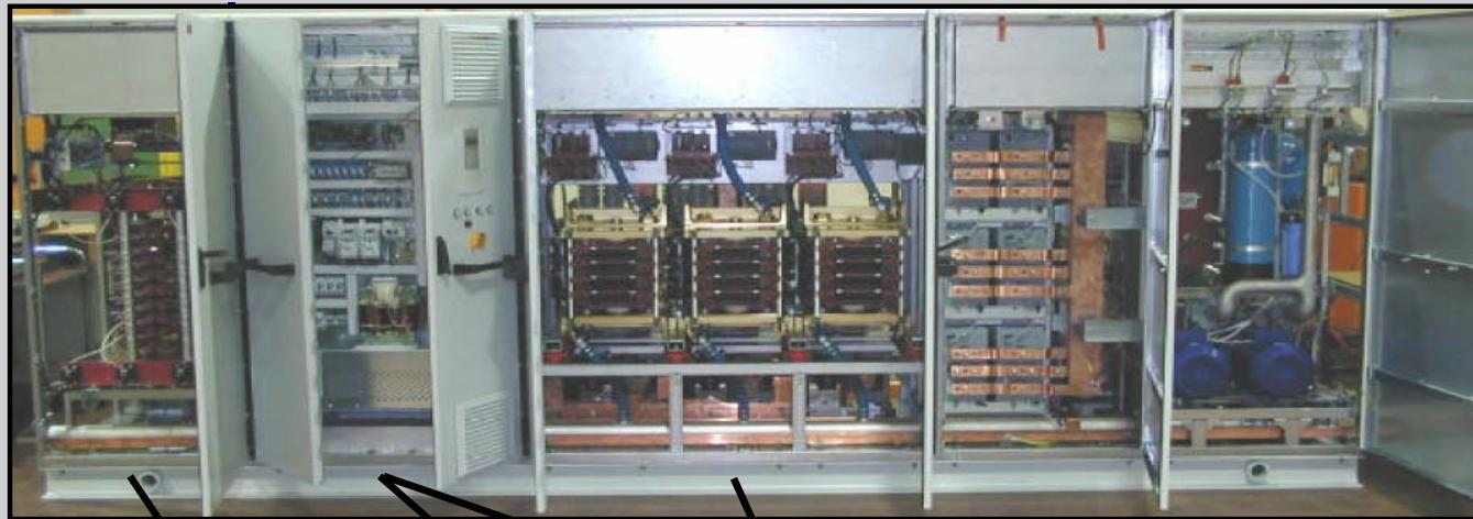
A medium voltage control unit for motor drives
